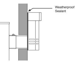
Feed the flue through the wall, making sure it runs smoothly.
