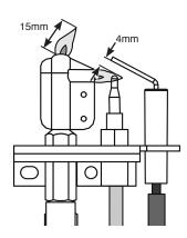
NOTE: Ensure the correct orientation when replacing.
