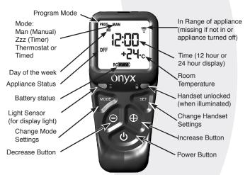
The lcon at the bottom of the screen displays the battery condition of both the batteries in the handset and in the Control Box alternatively.
