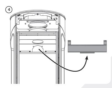
Note: When replacing the Main Baffle ensure that the Main Baffle flap rests on the Rear Baffle.
