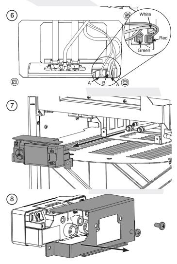
Replace in reverse order. Check all joints for gas leaks and check operation of the thermocouple and ignition lead.
