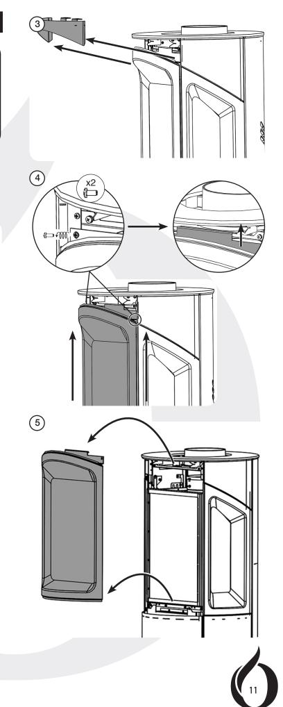
The glass frame must be refitted to the appliance following cleaning or servicing.
