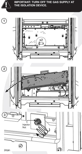
Extract the injector with the feed pipe from beneath the appliance.
