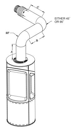
When A = 1.0 to 1.499 metres B+C = 1.0 metre max (Nat Gas - No restrictor, LPG - 75mm Restrictor) When A = 1.499 to 3.0 metres B+C = 4.0 metres max (Nat Gas - 70mm restrictor, LPG - No restrictor)
