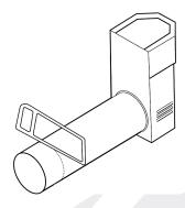
Terminal dimensions: 395 x 200 x 200 mm (H x W x D) Guard supplied Cut to length as required on site.
