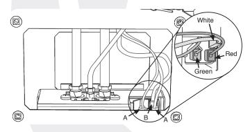
Gently withdraw the leads with Vidaflex through the base of the firebox.
