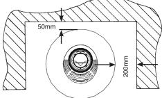
In a non-combustible recess be careful to allow enough clearance at the sides and rear of the appliance to perform spillage tests and reach the controls.
