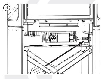
Connect a suitable pressure gauge to the test point located on the inlet fitting and turn the gas supply on. Light the appliance and check all gas joints for possible leaks. Turn the appliance to maximum and check that the supply pressure is as stated on the databadge. Turn the gas off and replace the test point screw, turn the gas on and check the test point for leaks.
