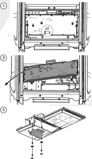
Replace with the correct size plate and secure the 2 nuts. Ensure that the lower edge of the plate is located over the venturi flange.
