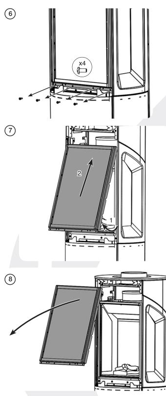
Replace ALL of the glass frame securing screws ensuring that a screw is present in all fixing slots.
