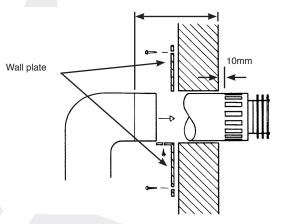
Measure from the outside of the wall to the stop on the 90° elbow.
