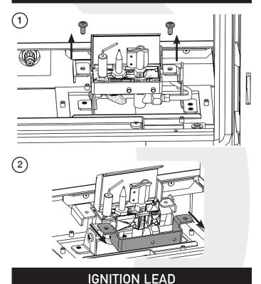
The Ignition Lead used on this appliance can not be replaced individually. If a new lead is required it will be necessary to
